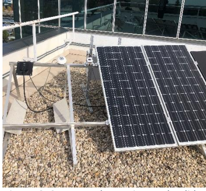
Figure 6. Set-up and experimental validation of the methodology to predict the energy output (monthly and annual daily average) of PV technology conducted at CEAETEMA of the University of Jaén. See refs. [62,63] for further details of the experimental set-up.
