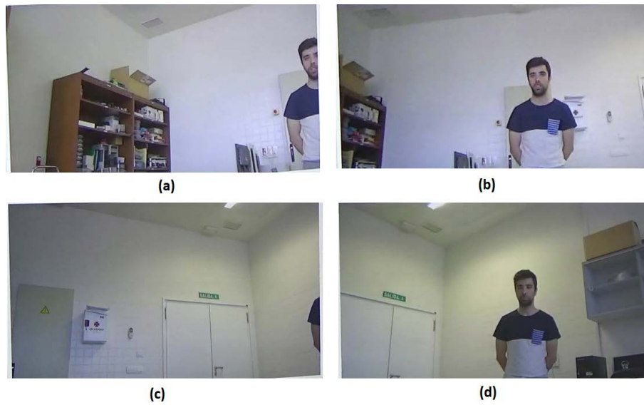
Fig. 10. Experiments. The figures depict the images of the monitor screen (a) Speaker has moved towards his left (b) The camera changes its orientation (c) Speaker moves again (d) The camera changes again its orientation
