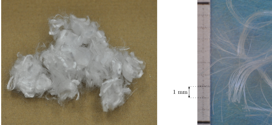
Figure 2: Polypropylene fibres used as reinforcement in the FRG specimens.
