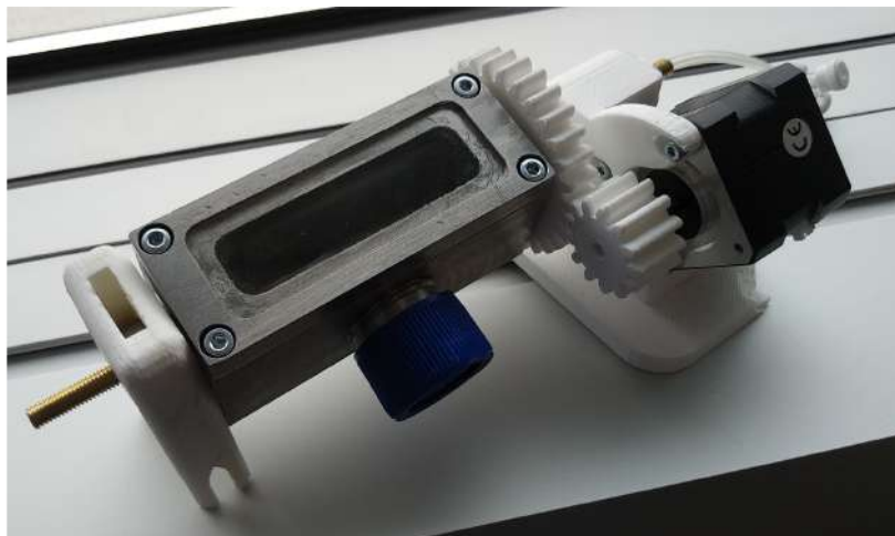
Figure 16. Photography of the bioreactor chamber
