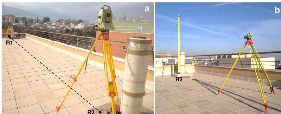
Fig. 4. Measuring the nominal values, horizontal distance (D) and height difference ( \Delta h ), between rover points R1 and R2 by using (a) Leica TCA2003 total station and (b) high precision leveling with a Leica DNA03 digital level and invar rods.
