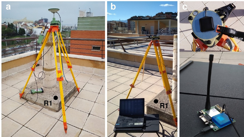
Fig. 2. Different instruments used in data acquisition: (a) Leica GS10 receiver and AS10 antenna on a surveying tripod, (b) u-Blox NEO-M8P GNSS antenna on a surveying tripod centered over the leveling benchmark and (c) Details of the NEO-M8P GNSS module and patch antenna.
