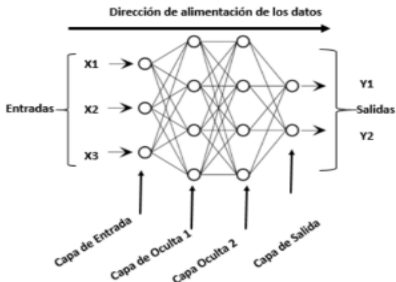
FIGURE 2.8: Topology of a Multilayer Perceptron by Valbuena, 2021. Model taken and edited from Hopgood, 2021.
