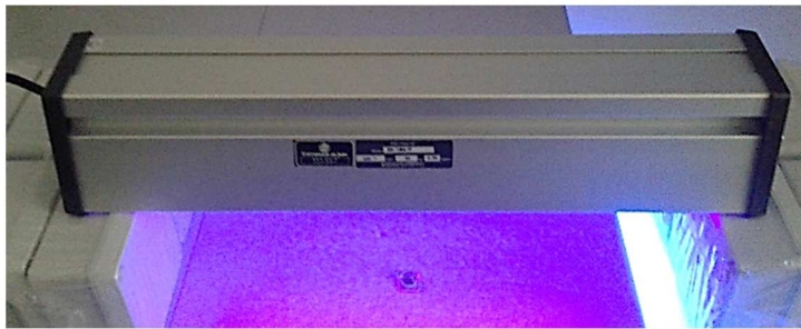
Figure 2. UV curing lamp, used for solidifying the optical adhesive between solar cell and refractive SOE, emitting UV light downwards over the receivers (SCA plus SOE).
