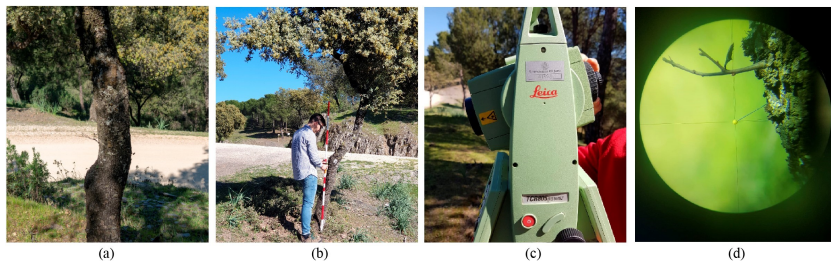
Figure 24 – Field measurements of structural parameters of trees. (a) The target tree, (b) The manually marking of the lowest point of the tree trunk, (c) Leica TCR-805 (TS), and (d) The view of the pointing to the pin on each side of the trunk.
