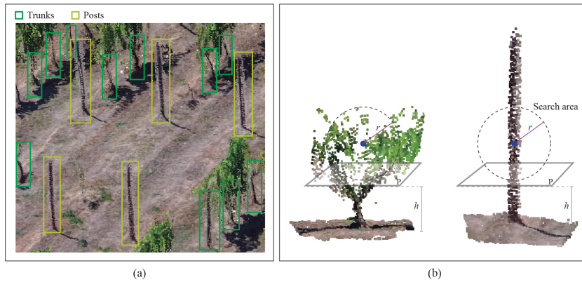
Figure 50 – Recognition of posts: (a) post location in the point cloud, and (b) the search of vegetation points around the trunk.
