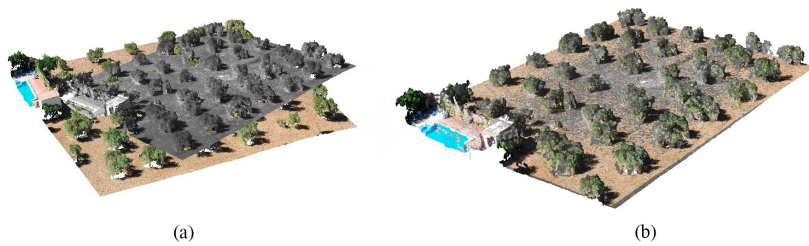
Figure 10 – 3D alignment: (a) initial position of point clouds, and (b) aligned point clouds.
