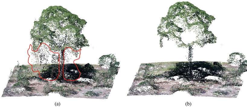
Figure 20 – The point-based filter of a cutout of the point cloud. (a) The original dense point cloud, and (b) The filtered point cloud.
