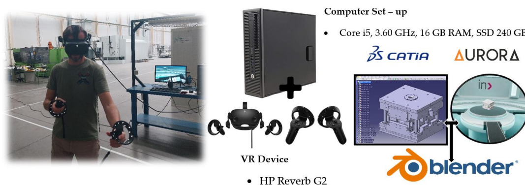
Figure 3. CAD – VR devices and environment.
