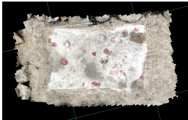
Fig. 4. Result of scanning with the “3D Live Scanner” application using the ToF technology. The result includes both geometry and image texture
