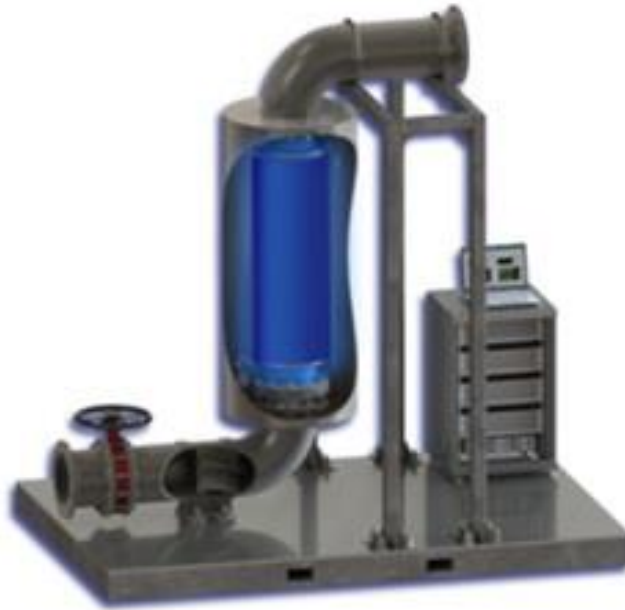
Figure 14 - Typhon treatment system reactor [14]
