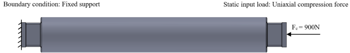
Fig. 3.- Boundary conditions and definition of the loads borne by the mechanical element.
