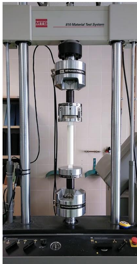
Fig. 9.- Uniaxial compression test of the mechanical element under study.
