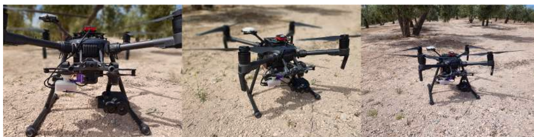
Fig. 2. Unmanned aerial vehicle, DJI Matrice 210 RTK, and thermal camera, DJI Zenmuse XT2, in the area of study.
