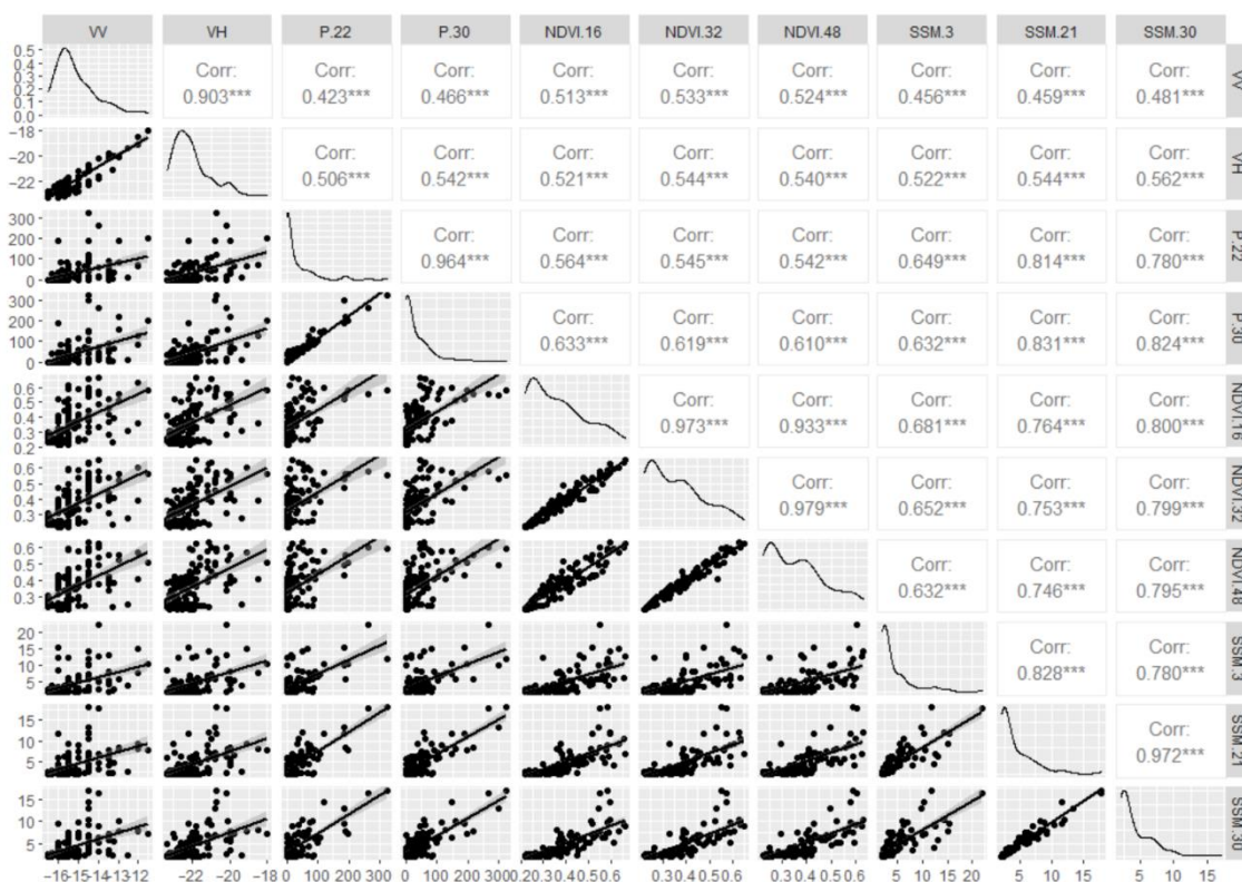
Figure 14. The correlation matrix of environmental variables, VV, and VH polarizations. Notes: charts on the matrix diagonal represent density distributions of values; charts on the top-right show linear correlation, characters “***” represent the significance of correlation at p < 0.001 ; charts on the bottom-left side present graphical scatter plots and linear regression models.
