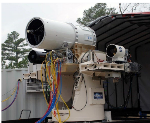
20 21 Fig. 7. Example of a high-power laser beam direction system for directed-energy applications 22 [121].
