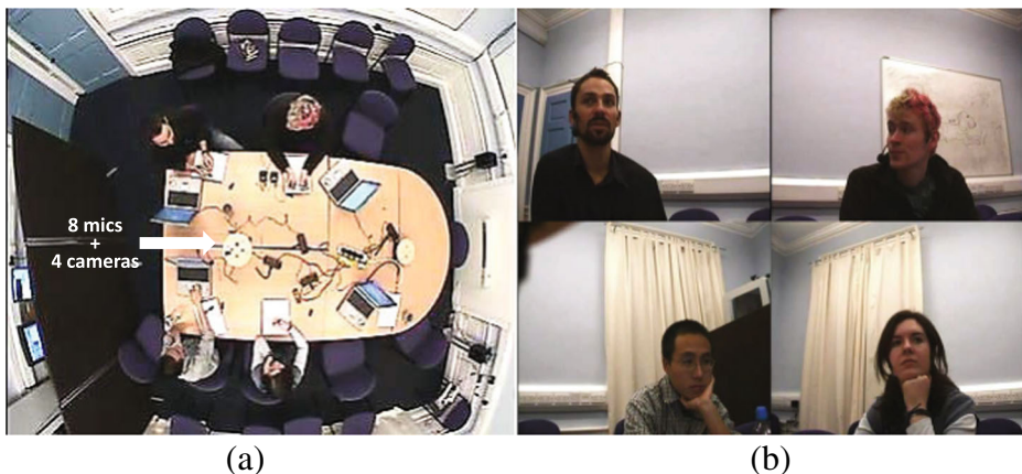
Fig. 1 a A meeting room included in the AMI dataset, equipped with an 8-channel microphone array and 4 cameras located at the centre of the table. b Video signals recorded with the cameras
