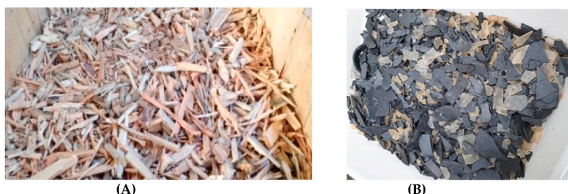
Fig. 5. Raw material used for joint gasification in the reactor. At left (A), pine-tree biomass. At right (B), WEEE, polyethylene and polypropylene.
