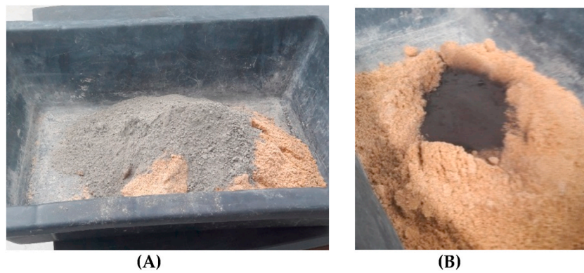
Fig. 8. Examples of the elaboration of mortar M1 (A) and mortar M2 (B), M3 is elaborated analogously to M2.
