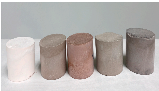
Fig. 4. Geopolymers samples: GMK; GMK-YC-BBA; GMK-RC-BBA; GMK-WC-BBA; GMK-BC-BBA.
