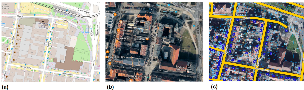
1 Examples of new cartographic products resulting from geospatial data integration (City of Poznań). a OpenStreetMap as an example of crowdsourced data, b Google Earth as an example of a web application, and c Cadastral parcel mapping as an example of integration between vector data and imagery (Source: http://poznan.podgik.pl/ ).
