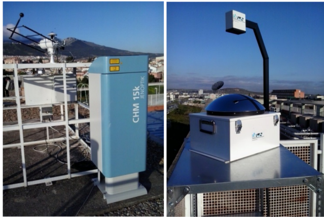
Figure 4.2: Meteorological station of the Univ. of Jaen. Left, Ceilometer and sun tracker in the background. Right, the TSI-880 sky camera.
